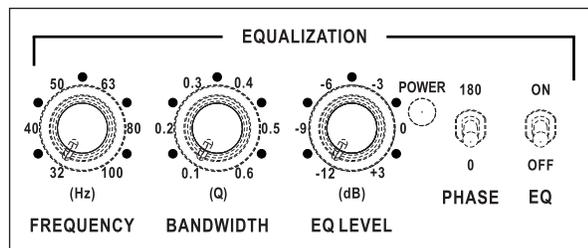
Figure 18: Equalization controls
