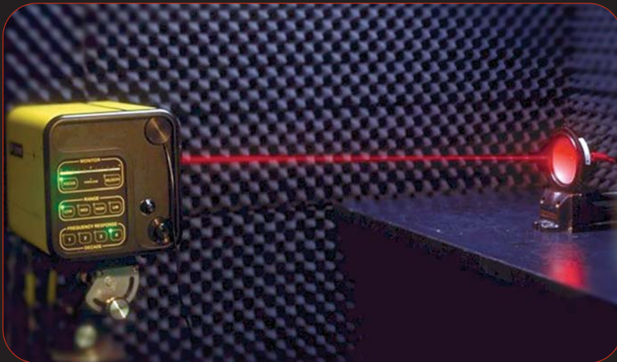
Laser interferometer scanning a transducer diaphragm
