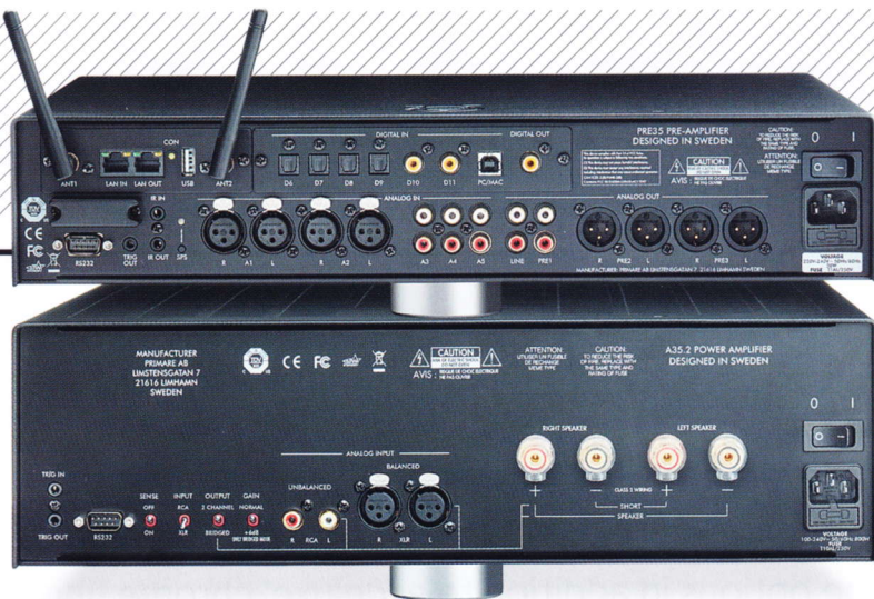
ABOVE: PRE35 [top] includes wired/wireless network streaming (Bluetooth, Airplay, Spotify, Chromecast) alongside a digital module (four opt, two coax and one USB-B), five line ins (two balanced on XLRs) and four analogue outs (two on XLRs). A35.2 [bottom] has balanced (XLR) and single-ended (RCA) ins plus 4mm speaker outputs
