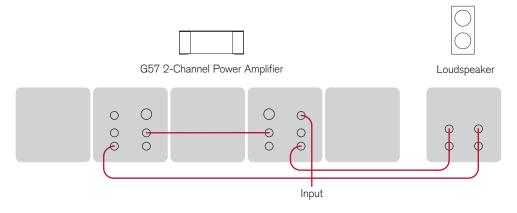
You can use the G57 as a mono power amplifier, to obtain more than twice the power output, by wiring it in bridge mode.
