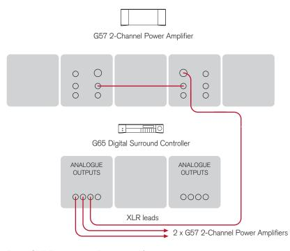
Three G57 Two-channel Power Amplifiers can be used in bridge mode for each of the front channels of a G65 Digital Surround Controller, which are provided as balanced outputs.
