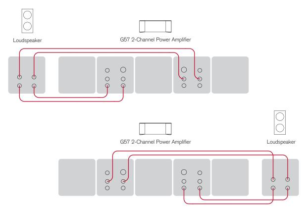
Extremely high sound quality can be achieved using two separate G57 Two-channel Power Amplifiers, one to drive each loudspeaker. The two channels in each G57 Two-channel Power Amplifier are used to drive the LF and HF units in each loudspeaker.
