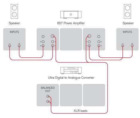
You can connect the Reference Two Channel Power Amplifier to a preamplifier with balanced outputs, such as the Meridian Ultra Digital to Analogue Converter.
