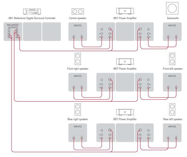
You can use three Reference Two Channel Power Amplifiers to drive the five loudspeakers and subwoofer in a surround system, using the six of the balanced outputs available on the OA18 cards.
