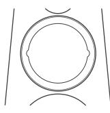
Hold the ring by one of the indentations by depressing the grille fabric with your thumb, and then wiggle the ring forwards until it comes free of the speaker. The grille fabric is very resilient and any depressions will soon disappear.
