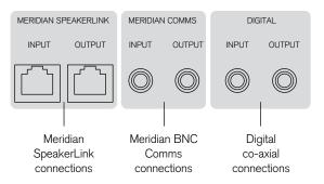
You can connect to the DSP loudspeakers using either the SpeakerLink connectors, or the Meridian BNC Comms and digital co-axial connectors.
