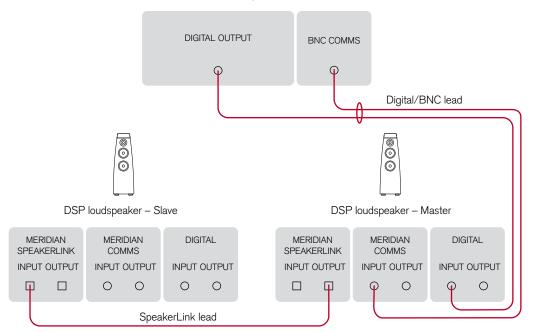
If the Meridian source or control unit provides a Meridian BNC Comms output, you will need to connect it to the DSP Loudspeakers using a Digital/BNC lead.
