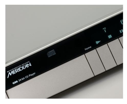
DAC rated at 192 kHz, 24-bit for maximum analogue performance
