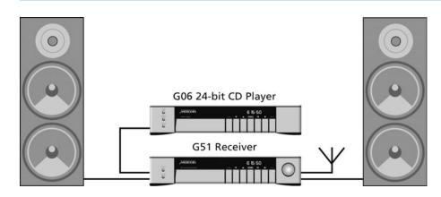
The player utilises 192 kHz, 24-bit digital to analogue converters for the very highest analogue quality, while the internal circuitry includes a superb analogue design to complement the high-spec DACs and delivering 2V rms with less than –95dB noise and distortion.
