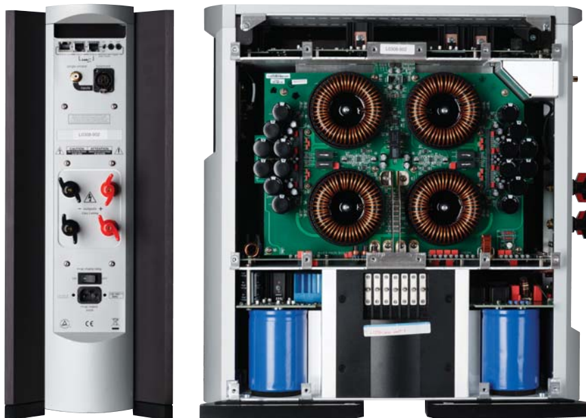
This side view shows the four different compartments of the amplifier: the power supply section at the bottom, the middle section with the four amplifiers, the top section with the control circuitry (modulator), and a separate enclosed box (top left) that houses the analog input board.
