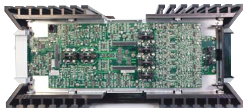
The modulator board is the "brain" of the system. It is located at the top of the amplifier in order to provide shielding from the main amplifier section.
