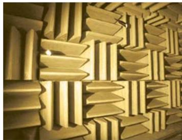
72 frequency response measurements are taken at different points around the loudspeaker, in one of four anechoic chambers. This allows for accurate analysis of a speaker's total performance before the listening tests even begin.
