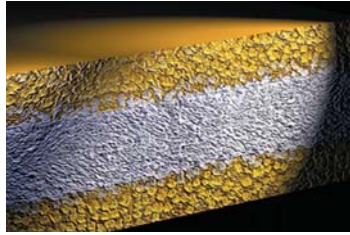
CMMD cones consist of a stiff aluminum core, deep-anodized on both sides (alumina) for increased strength and rigidity.
