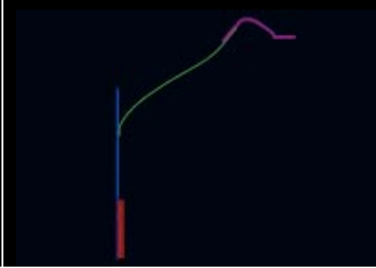
Figure 7. The shape of the first mode with a paper cone, at 2160Hz.
