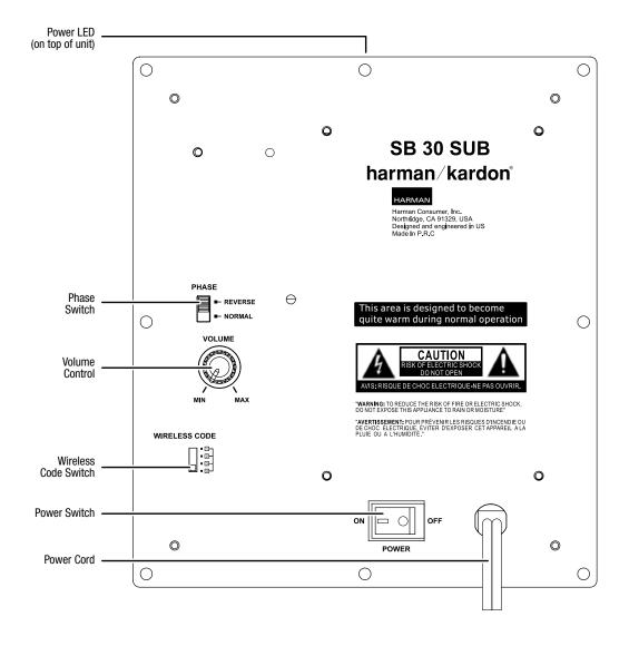
Power LED (on top of unit): The Power LED's color indicates the subwoofer's operational status:
