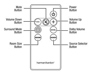
Mute button: Press this button to mute the system (the soundbar Power LED will flash blue); press again to unmute the system.
