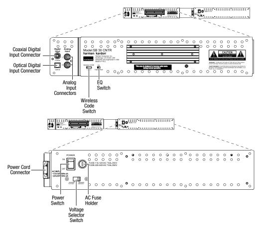
Coaxial Digital Input connector: If your TV, disc player or cable/satellite tuner has a coaxial digital output, use a coaxial digital audio cable (not supplied) to connect it here.
