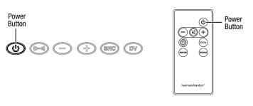
**NOTE:** If you put the soundbar into the Standby mode manually, you can turn it back on only by manually pressing the Power button again.
