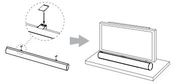
As long as the table's surface is flat, the soundbar will rest on the rubber feet.
