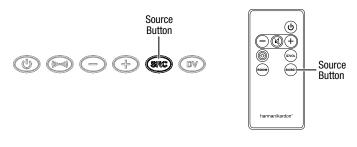
The soundbar's Status LEDs will glow white to indicate the active source.
