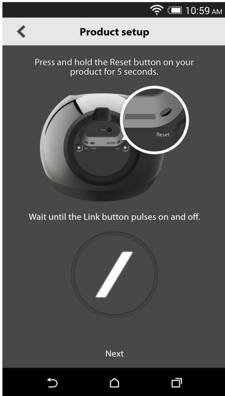
Follow the on-screen instructions. First connect your product to power and turn it on. Wait several seconds for the unit to power on completely, then press and hold the 'Reset' button on the bottom panel of the unit for 5 seconds. The Link button LED will flash quickly for several seconds, then begin to pulse slowly. After this, flick the screen to the left. This will display the next step.
