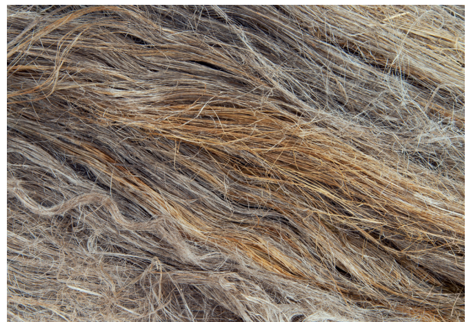
Flax offers unique qualities: light because it is hollow and very low elasticity. It constitutes a choice suitable for the manufacture of the core of a sandwich structure.
