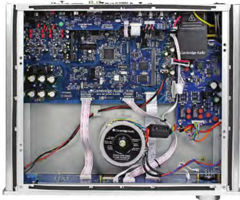
Inside, the Cambridge 851N uses a beefy toroidal transformer in its power supply. And just look at all those heavyweight digital chips...
