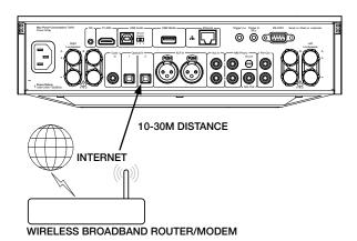
Place the Evo 75/Evo 150 in range of your wireless network (usually 10-30m of a suitable wireless transmitter, although this is affected by walls and the construction of your building) and turn it on, via the back panel switch and then on the front panel
