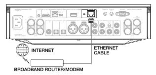
Plug one end of a network cable (Category 5/5E straight through Ethernet cable) into the LAN port on the back of the unit.
