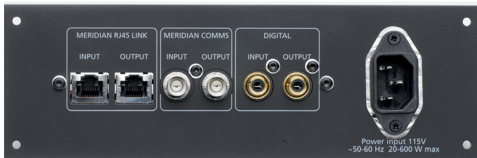
DSP7200 rear panel showing RJ45 connectors.
