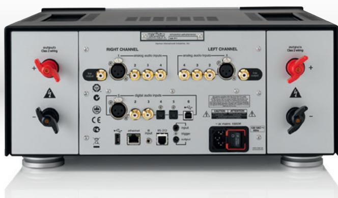
△ THE REAR PANEL IS A POSTER-BOY FOR ORGANISED LAYOUT, WHILE THE 'HURRICANE' BINDING POSTS ARE AMONG THE BEST IN THE BUSINESS.
