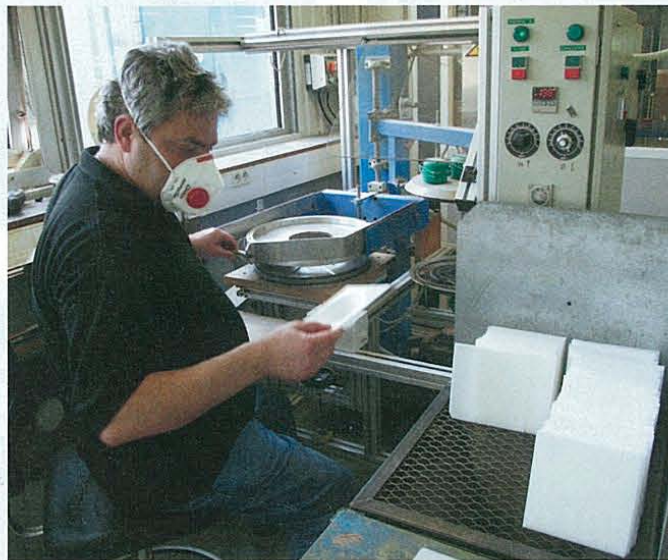
A technician forms flat Rohacell foam wafers (white squares at right) into cones.
