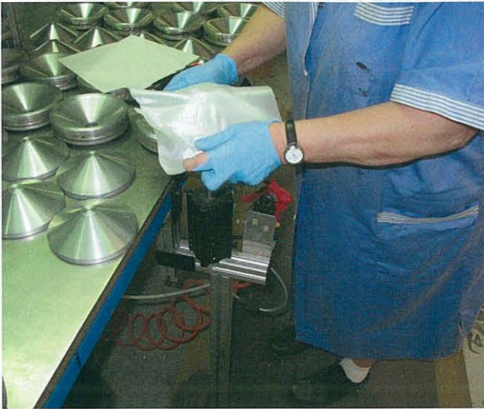
A technician stretches resin-impregnated glass-fiber sheets over the Rohacell core to form Focal's "W" composite-sandwich diaphragms.
