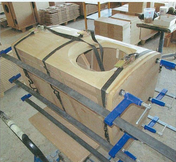
A Stella Utopia EM woofer enclosure under construction.
