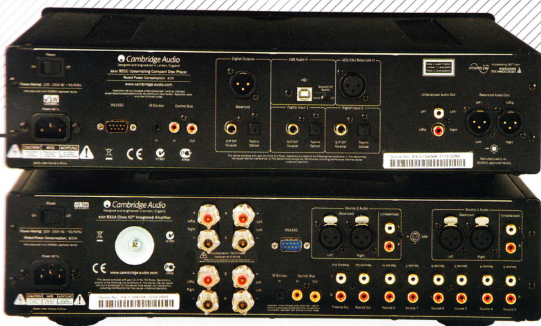
ABOVE: Matching balanced (XLR) and single-ended (RCA) connections are joined by a suite of USB and S/PDIF inputs on the player with two sets of speaker outs on the amp
