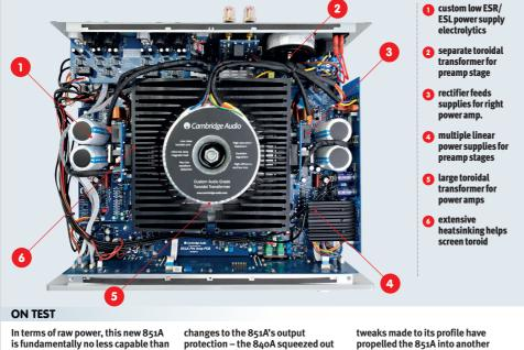
changes to the 851A's output protection – the 840A squeezed out 485W/20hm while the 851A is 'limited' to 310W/20hm. With any sane loudspeaker this is unlikely to make a practical difference. The lower 0.030hm output impedance of the 851A and wider 91dB A-wtd S/N ratio (re. odBW) are, however,
