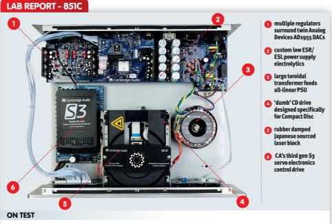
Whether used for CD replay or as an outboard DAC with another digital transport or USB service, the 851C offers a remarkably high and consistent performance. The balanced (XLR) outputs are set to 4.3V from a usefully low 450hm source impedance while all sources (CD/digital) benefit from a wide 112.5dB A-wtd S/N ratio. This includes USB which maintains a true 24-bit performance up to 192kHz with no
