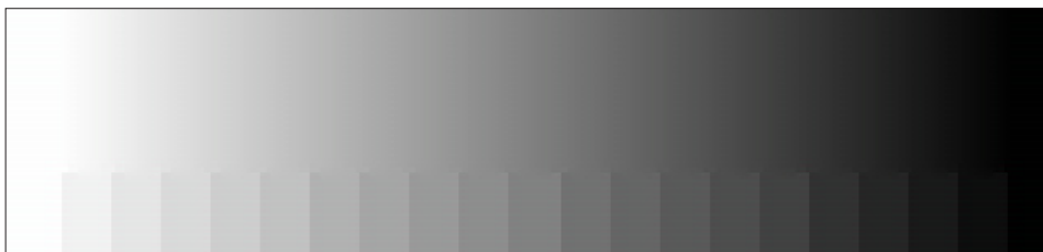
Figure 11: Gray scale ramp image AFTER Qdeo True Color processing. The banding in the top portion of the image has been removed while preserving the sharpness of the steps in the bottom portion of the image.
